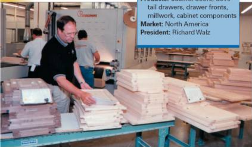
Richard Walz, president of WalzCraft Industries, inspects cabinet doors before going through a Timesavers five-head custom-built widebelt sander.
