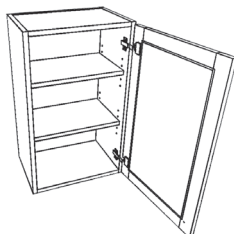
Hinge Boring on Right Stile Hinge Bore Location = R
