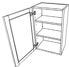
Hinge Boring on Left Stile Hinge Bore Location = L
