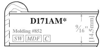
D171AM* Molding #852 SW MDF C PC: AM101 Multiplier: .70 No Hinge Boring Available
